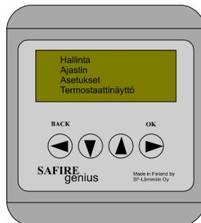
Place the control panel so that the display is easy to see and use, and that there's no danger of starting the heater by accident. Both control panels can be either surface or flush mounted. Attach the control panel to the connector inside the heater (remove the base of the heater). 1600D heater: the control panel cable replaces the heater's own control panel cable.
